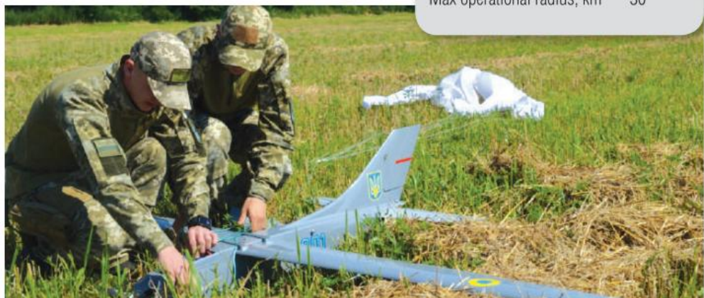
The Spectator-M is a hand-launched, T-tail high-wing monoplane (parasol) constructed mainly of composite materials
