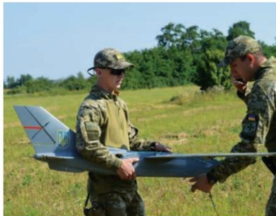
The Spectator-M is a hand-launched, T-tail high-wing monoplane (parasol) constructed mainly of composite materials
