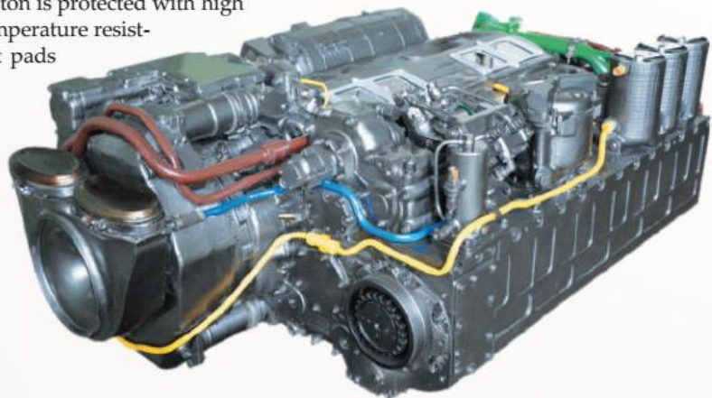
The 6TD-2 is the most popular engine among all TD-series engines produced by Malyshev Plant
